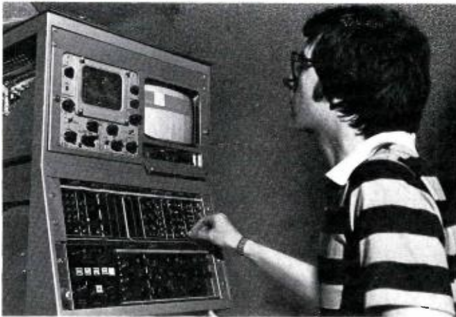
Video module includes control units for three TKP-45's and three TK-44 cameras.
