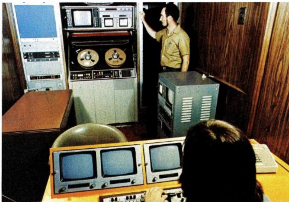
Fully equipped recreational vehicle is used for location shoots. Unit is equipped with a TKP-45 camera; TR-600 VTR; video switching and audio facilities, and a 6 kW generator.
