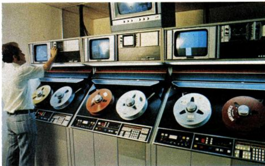
TR-600's are set up for three-machine editing. Both local and remote editing control panels are installed for added flexibility.
