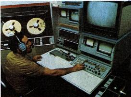
Master Record facility next to the studio area is equipped with a TR-600 tape machine; camera control units, and a basic video switcher.
