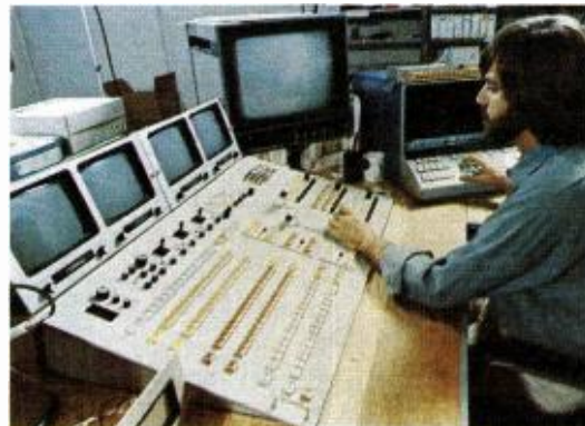
Editing and dubbing area includes three TR-600's, video switcher and computer editing system. Facility operates around the clock during the week to handle dubbing requirements.
