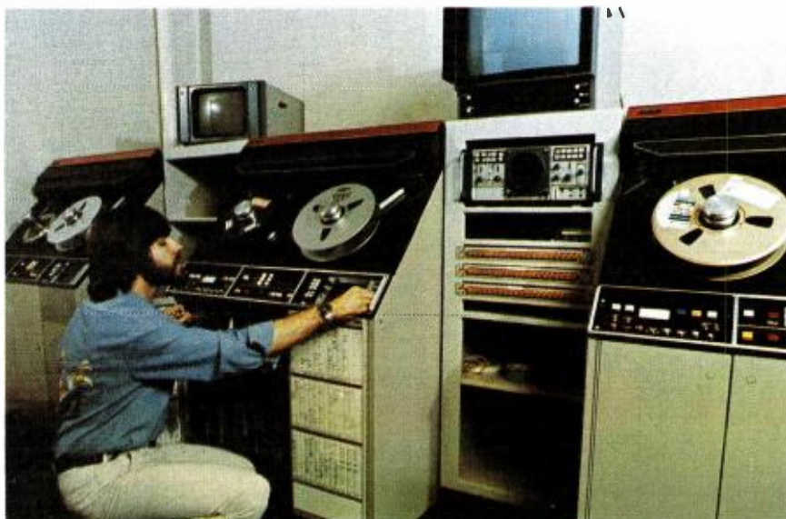
Editing and dubbing area includes three TR-600's, video switcher and computer editing system. Facility operates around the clock during the week to handle dubbing requirements.
